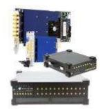
Among our 130 different digitizers, you will find the bestsellers of the "22" series. These 8-bit digitizers offer ultra-fast sampling rates from 1.25 GS/s to 5 GS/s and bandwidths from 500 MHz to 1.5 GHz. A total of 34 different models are available as PCle & PXle cards (1 to 4 channels) or LXI/Ethernet standalone units (2 to 24 channels).
