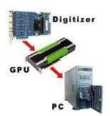
With digitizers and AWGs, there is often a bottleneck in processing the large amounts of data. Spectrum Instrumentation solves this problem with the "SCAPP" option, using a CUDA graphics card between the instrumentation card and the PC. The GPU of the graphics card, with up to 5000 cores, provides much faster parallel processing than the CPU of the PC with only 8 or 16 cores.
