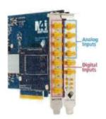
For mixed-signal testing, a piggyback module provides 8 additional digital input lines for SPECTRUM's popular high-speed and high-resolution PCle digitizers of the "44"-series (14 bit with up to 500 MS/s). Analog and digital inputs work fully synchronous.
