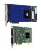
With 32 channels and clocking speeds up to 720 MHz, Spectrum's M4i.77xx series of Digital Acquisition cards make pattern recognition and logic analysis fast and economical. Differential or Single-Ended inputs are available! The brand-new Digital I/O card M2p.7515 also offers 32 channels with speeds up to 125 MHz, making it perfect for cost-effective pattern recognition and generation.
