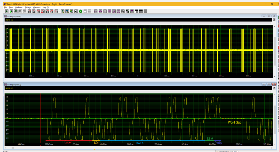
Figure 1: A two second record of an ARINC429 differential signal acquired using a 1 MHz acquisition clock shown in the top grid. A horizontally expanded view in the lower grid shows the bipolar return-to-zero format and is annotated to show specific data.
