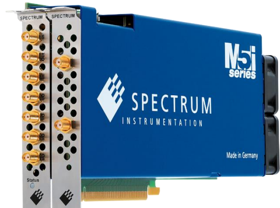
Fig. 2: The M5i.3321-x16 digitizer card offers 3.2 GS/s sampling speed, 12 bit resolution and 1 GHz bandwidth on each of the two channels. The M5i.33xx family has 5 different models with 10 GS/s top speed and over 3 GHz as highest bandwidth.
