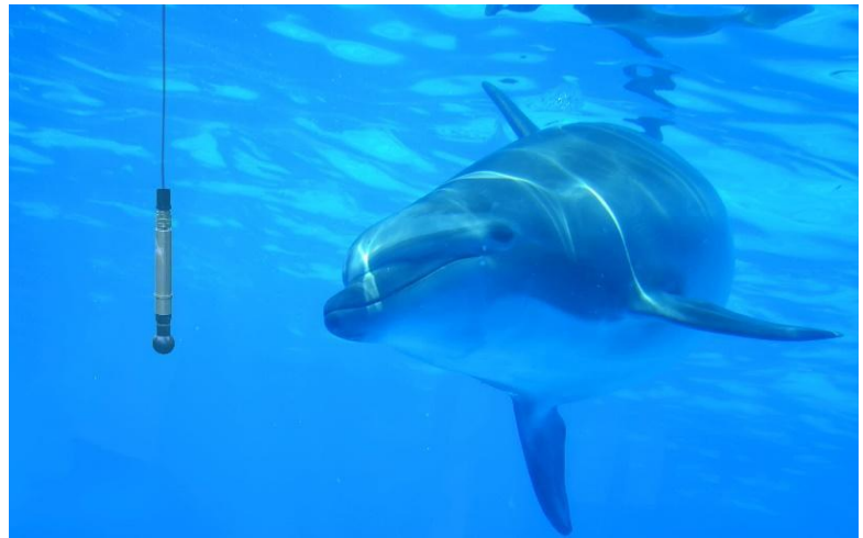
A combination of hydrophones, digitizers and a custom-developed AI is able to locate the focus of the dolphin's sonar clicks.
