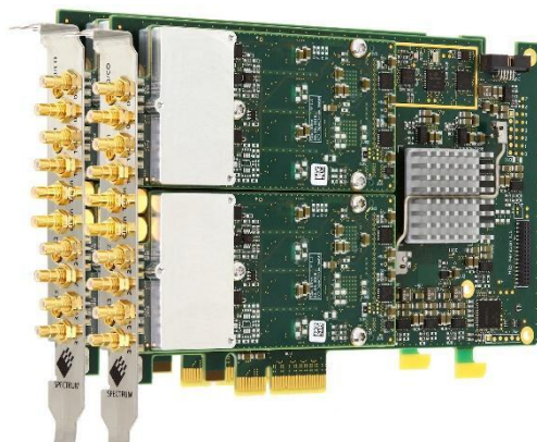
Two M2p.5913 digitizer cards provide 16 acquisition channels using only two PCIe slots. The M2p.59xx series by Spectrum Instrumentation offers 24 different card variants with 5 to 125 MS/s sampling speed, 1 to 8 channels per card and 16-bit resolution.
