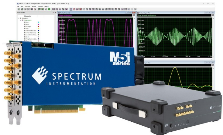
offer one or two channels with up to 10 GS/s output rate, 16-bit resolution and 3.9 GHz bandwidth.
