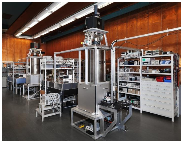
The two caesium fountain clocks at PTB provide the legal time for the entire Federal Republic of Germany. (Photo courtesy of PTB)
